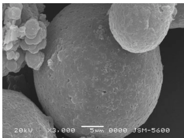
Figure 1 SEM micrograph of poly(HPMA-GMA) gel beads.
